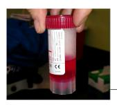
This is a vial of Enteric Transport Media (ETM) that is used for enteric pathogen, norovirus, and parasitic Cryptosporidium\* testing.
