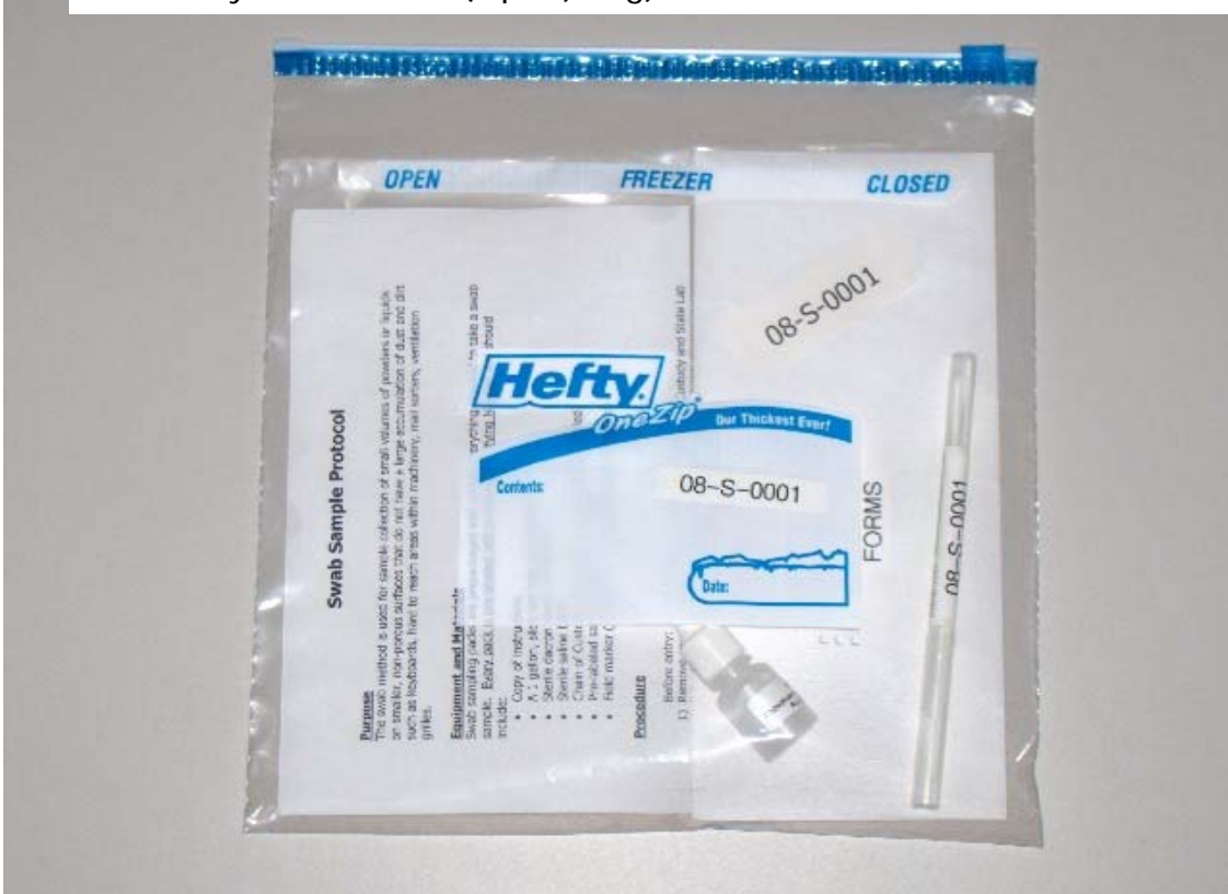
Pictures show one swab sample kit complete with: Sampling Protocol, State Lab and Chain of Custody Forms, sterile swab, saline bottle, secondary containment (Ziploc) bag), and field location marker.
