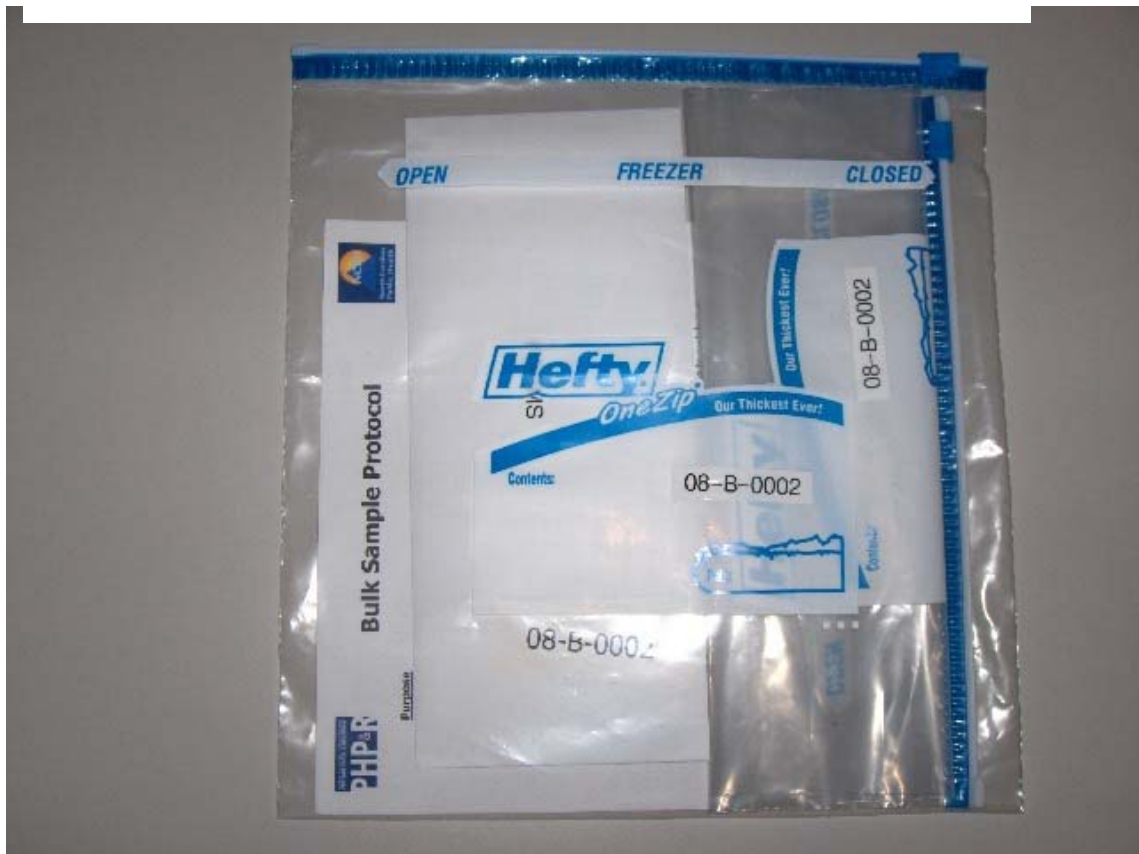
Pictures show one bulk sample kit complete with: Sampling Protocol, State Lab and Chain of Custody Forms, Primary and Secondary Zip Lock bags, and field location marker.
