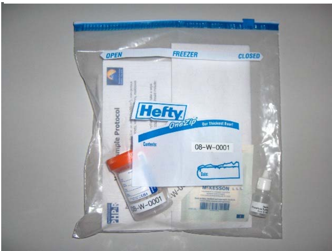
Pictures show one wipe sample kit complete with: Sampling Protocol, State Lab and Chain of Custody Forms, sterile specimen cup, saline bottle, sterile 2x2, secondary containment (Ziploc) bag, and field location marker.
