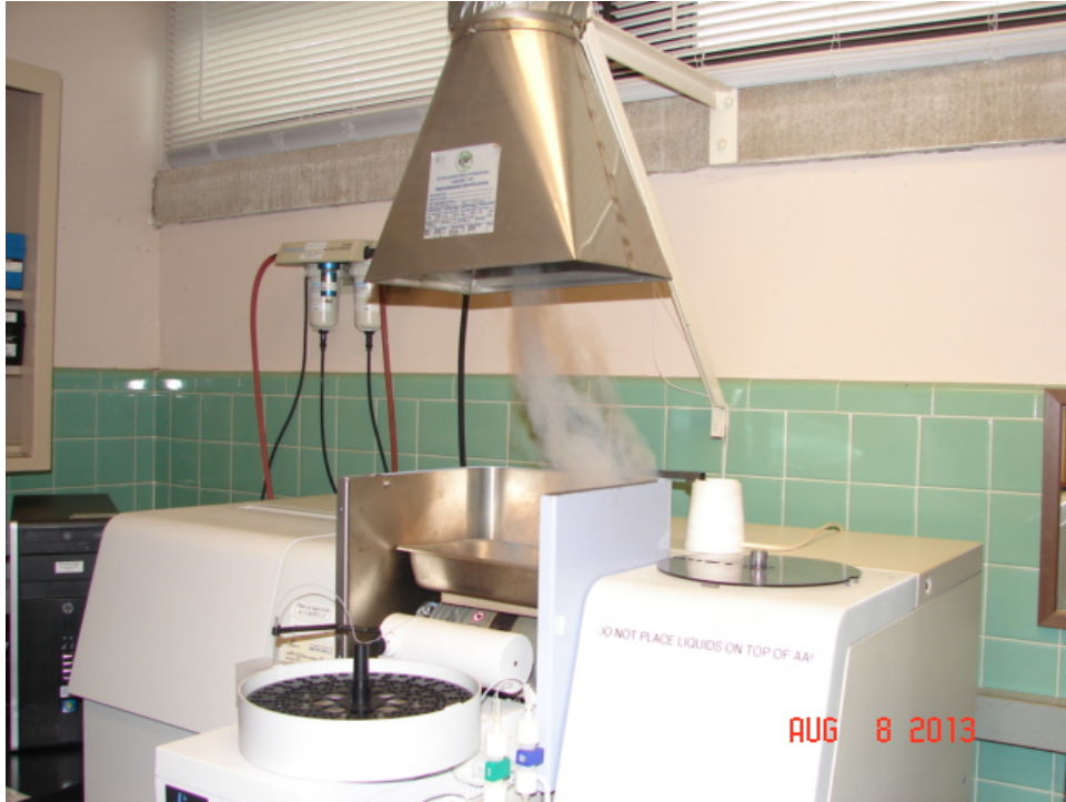
Figure 1: Smoke test of Atomic Absorption Spectrophotometer (AAS) Hood
