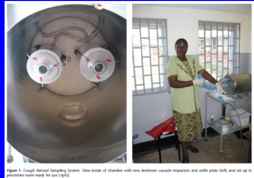
Figure 1. Cough Aerosol Sampling System. View inside of chamber with two Andersen cascade impactors and settle plate (left) and set up in procedure room ready for use (right).
