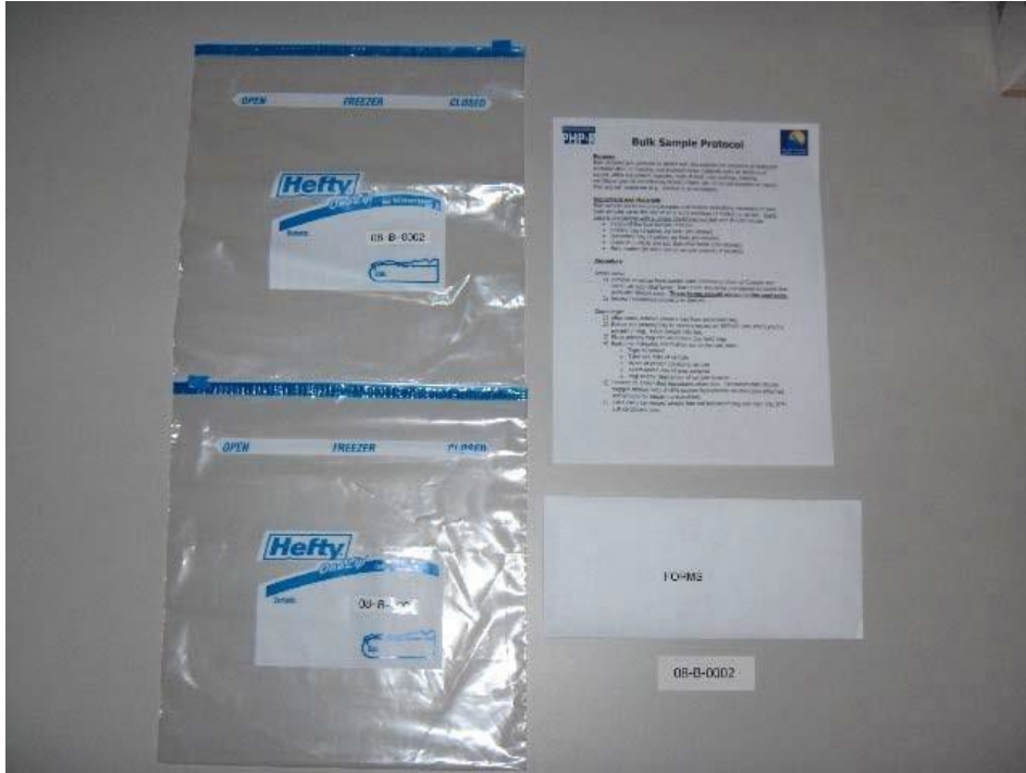
Pictures show one bulk sample kit complete with: Sampling Protocol, State Lab and Chain of Custody Forms, Primary and Secondary Ziploc bags, and field location marker.
